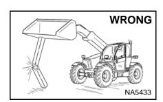
Never work on telescopic handler with boom up unless boom is held by an approved boom stop. Replace if damaged. Never modify equipment or add attachments not approved by **Bobcat Company.**
