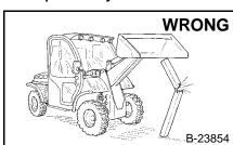
Never work on the machine with lift arm up unless supported by an approved support device. Replace if damaged. Never work on a raised implement unless it is properly supported.
