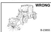
Disconnecting or loosening any hydraulic tubeline, hose, fitting, component or a part failure can cause lift arm or implement to drop. Do not go under lift arm when raised unless supported by an approved lift arm support device or under raised implement without proper supported. Replace if damaged.
