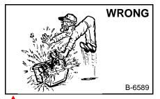
Lead-acid batteries produce flammable and explosive gases.
