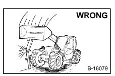
Never work on VersaHANDLER with boom up unless boom is held by an approved boom stop. Replace if damaged.
