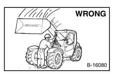
Disconnecting or loosening any hydraulic tubeline, hose, fitting, component or a part failure can cause boom to drop. Do not go under boom when raised unless supported by an approved boom stop. Replace if damaged.
