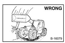
Never work on VersaHANDLER with boom up unless boom is held by an approved boom stop. Replace if damged.
