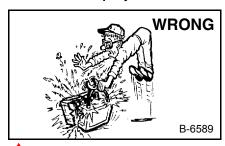
Lead-acid batteries produce flammable and explosive gases.
