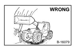
Never work on VersaHANDLER with boom up unless boom is held by an approved boom stop. Replace if damaged.
