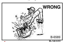
Lead-acid batteries produce flammable and explosive gases.
