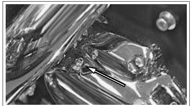
Figure 1-3. Actuator Bleeder Valve (plastic cap removed)
